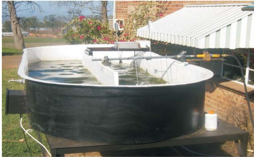
*Figure 6 Experimental micro-algae production system*
