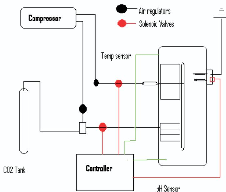
Figure 5 Schematic layout of micro-algae production system
