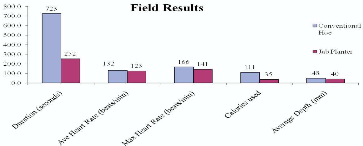
Figure 4 Performance of maize planting using a conventional hoe and jab planter
