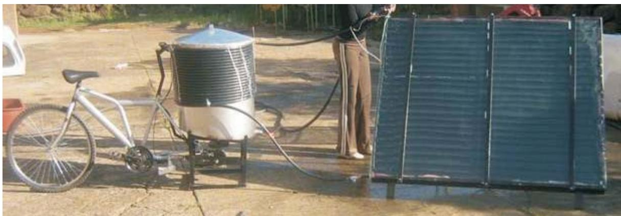
*Figure 9 Human powered honey extractor and heating system*
