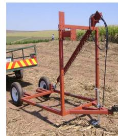
Figure 1. *Trailed implement frame with de-trashing device attached*
