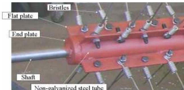
Figure 3. De-trashing device
