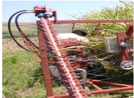
Figure 4. Mounting of de-trashing and topping device
