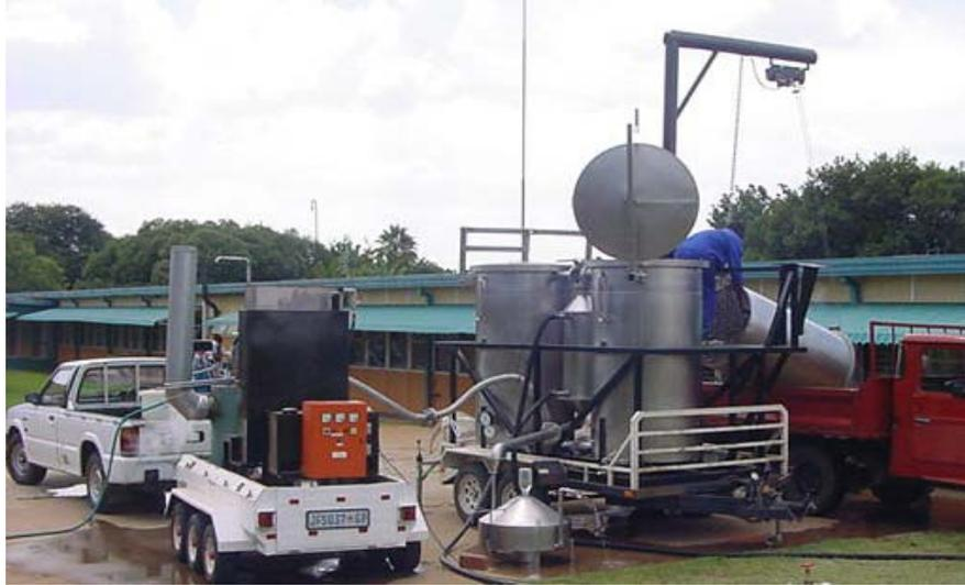
*Figure 1. Mobile essential oil distillation unit in operation.*
